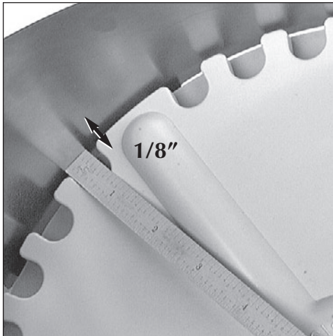
Fig. 26 - Make sure the casefeed plate is centered in the bowl with approximately 1/8" all the way around.
