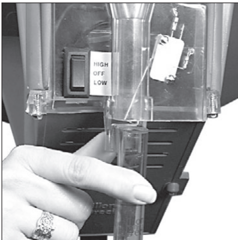
Fig. 8 - The end of the casefeed tube marked "up" snaps into the clip at the base of the casefeeder motor housing.
