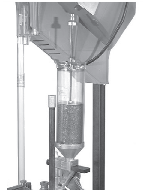
Fig. 25 - Dillon's Low Powder Sensor gives an audible and visual warning when the powder reservoir gets low.
