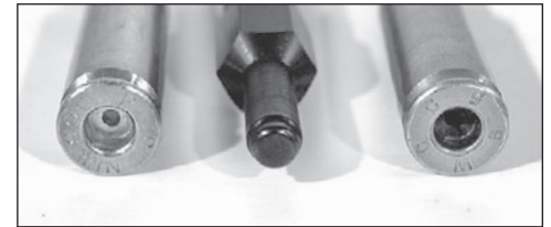
Fig. 59 - Note the difference between the swaged primer pocket (left) and the unswaged primer pocket (right).
