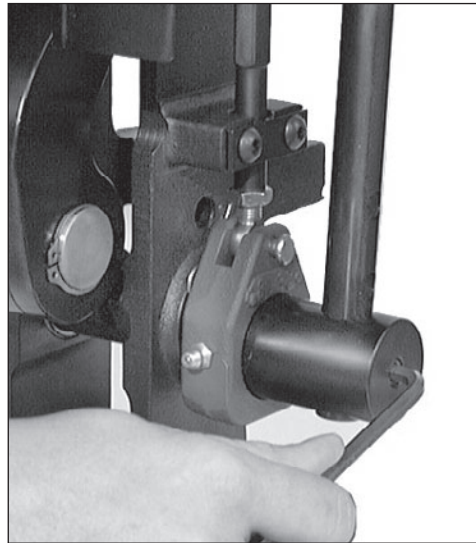
Fig. 2 - Note that there are three different positions for mounting the operating handle.
