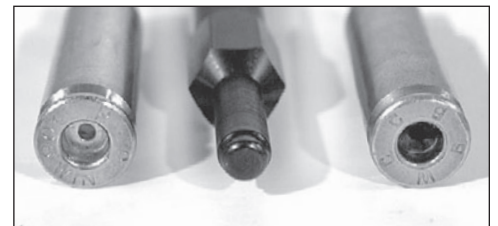
Fig. 31 - Note the difference between the swaged primer pocket (left) and the unswaged primer pocket (right).
