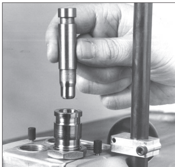
Fig. 18 - Drop the powder funnel into the powder die tapered end first. The funnel should move freely in the die.
