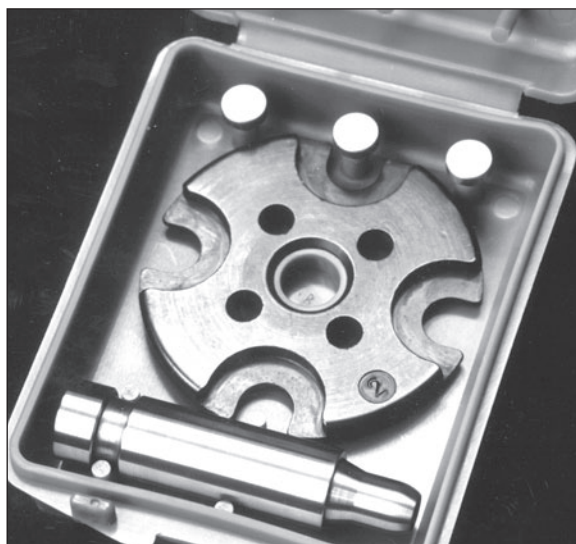
Fig. 4 - This photo shows a complete caliber conversion; the powder funnel, shellplate and locator buttons.
