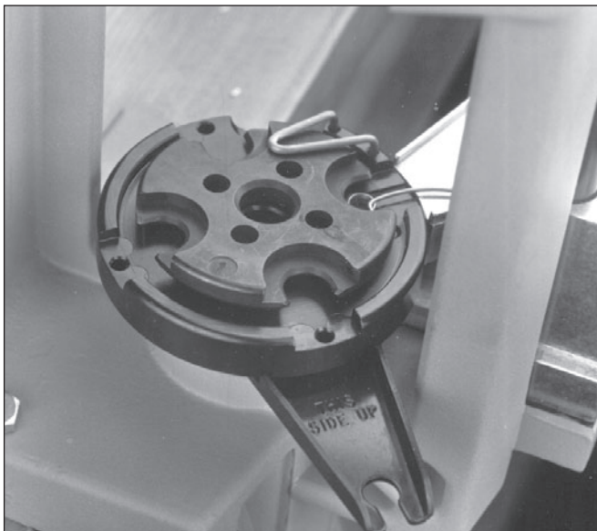
Fig. 6 - Showing the shellplate in its proper position: under the ejector wire with the shellplate number up.
