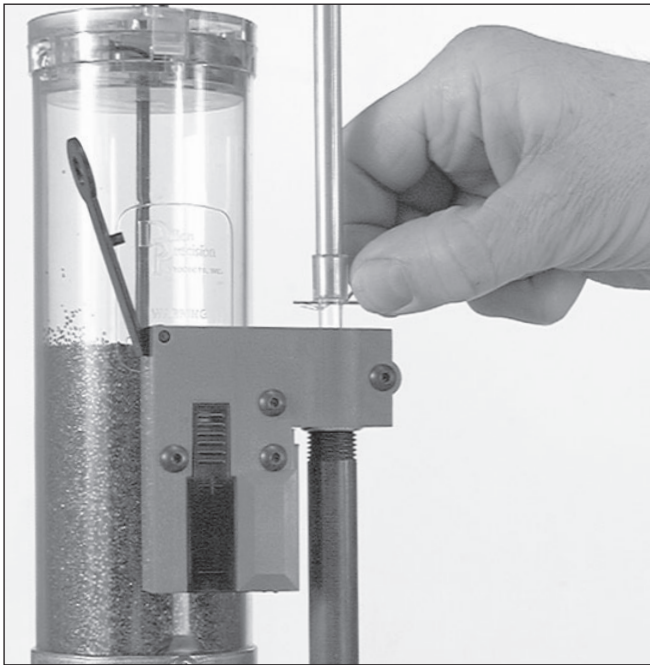
Fig. 26 - Drop the primers into the primer magazine.
