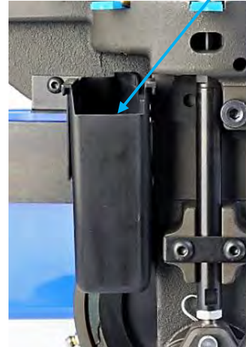
Spent Primer Cup—Slides onto Bracket
