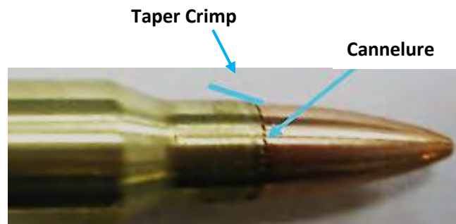
Taper Crimp of Rifle Cartridge with Cannelure
